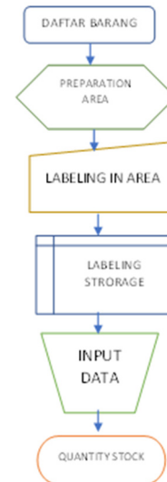
Gambar 3. Bagan Alur Sub sistem Warehouse
