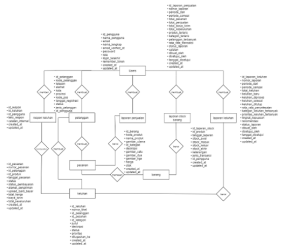
Gambar 4. Entity relationship diagram (ERD)
