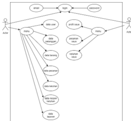
Gambar 3. Use case diagram
