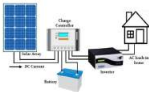
Gambar 1. PLTS Off Grid
